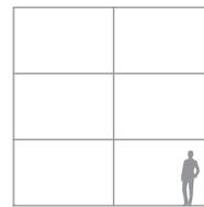
The facade system consists of 6 mullion/transom profiles with a reduced size of only 50 mm. Available in three materials (galvanised steel, stainless steel and Corten steel) they have different lengths, up to 8 m and depths, from 50 mm to 180 mm. By increasing the depth of the profile, it is possible to increase the dimensions of opaque and glass panels up to approximately 7 sqm, thus giving the designer the possibility to choose the profile that best matches their project needs.
