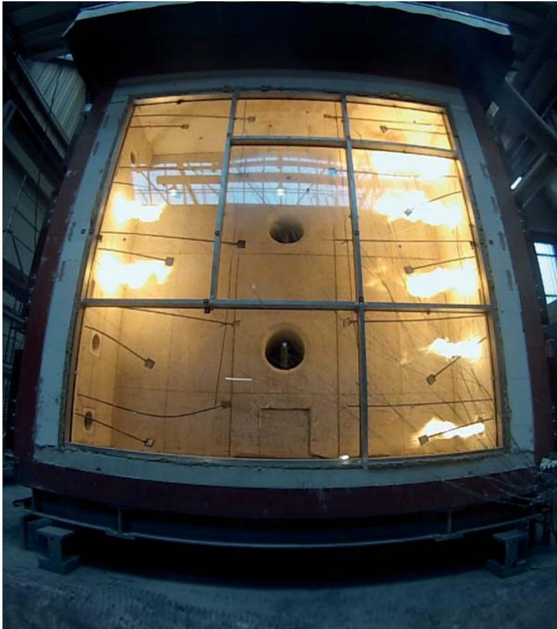
Fire-resistant elements and components have been specifically designed to meet the requirements of structural resistance and internal temperatures of 1000° C, retention of external surface temperatures below 180° C, absence of hot flammable fumes, dimension and weight of glasses that can reach huge proportions, duration of performance levels up to 90 minutes.
